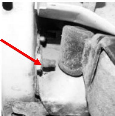
40. Install the new spring packs with the factory hardware removed in step 27. It is a good idea to grease the threads on the spring bolts. Mount the frame end first and then the shackle. Install the supplied pair of 6 degree axle shims and new centering pins to install to the leaf springs if needed in order to obtain the proper driveline angle. (Note: Do not torque hardware until instructed.)
